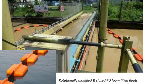
Rotationally moulded & closed PU foam filled floats with nominal thickness of 4-6mm and corner exceeding 8mm provide great structure I integrity make it impact resistance and long lasting
